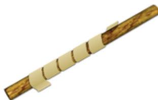
Figure 51: A Scytale, an early device for encryption
