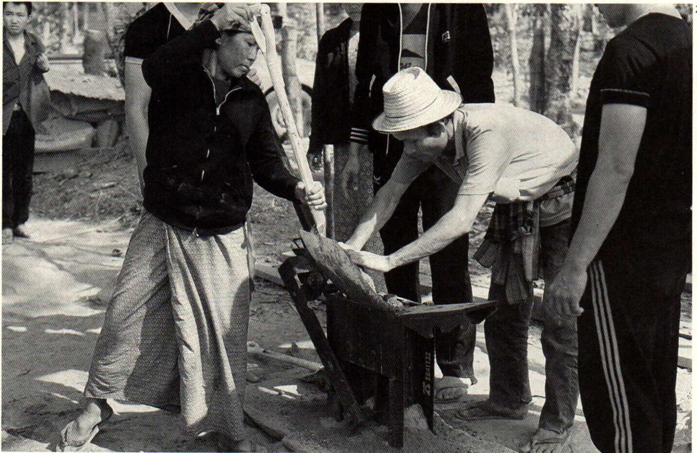
2. Mixed soils are placed in the pressing block. This machine is easily operated by rural people.
