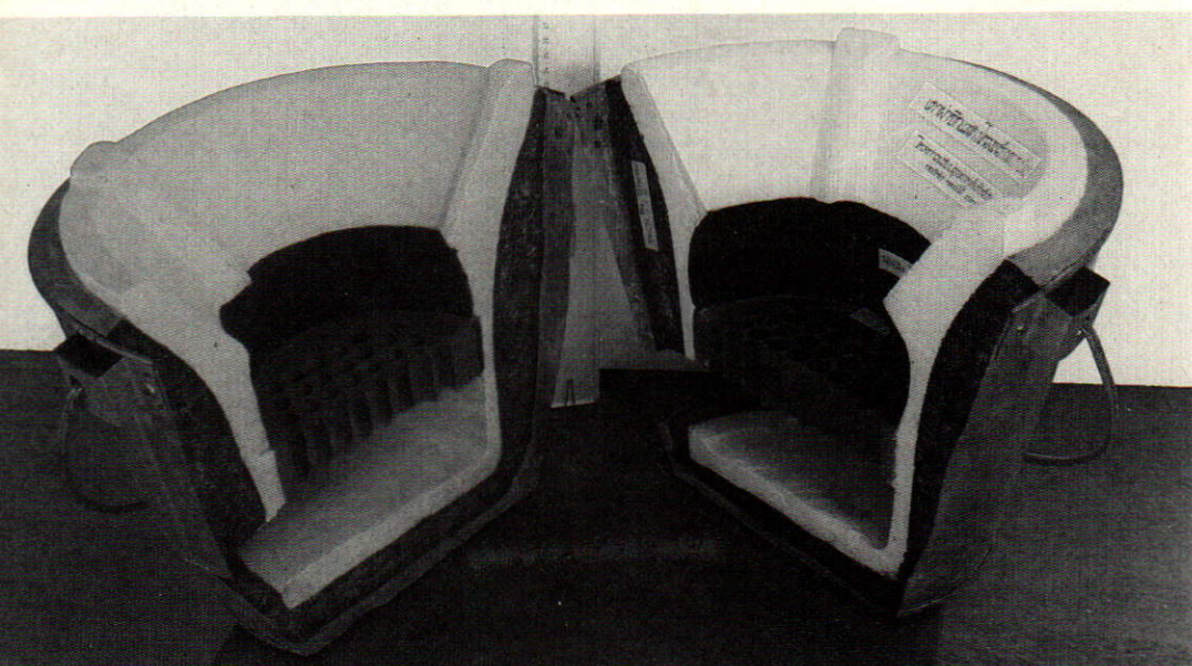
6. The improved design model "RFD-1" charcoal stove development under USA-RTG Technical Co-operation on Renewable Non-conventional Energy Project. The peak heat utilization efficiency under laboratory test is 32-34% at charcoal load 400-500 gm. The pottery liner is heat refractory.
