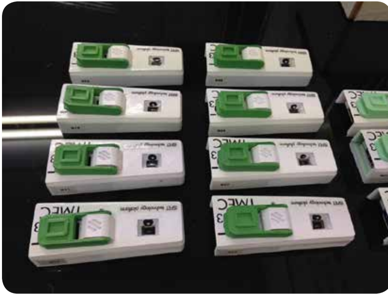
The nitrate sensor based on ISFET Technology
