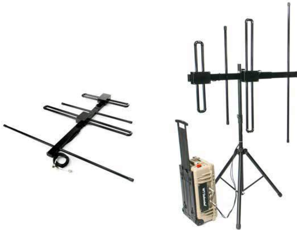
Antenna installation with Walkie-Talkie Jammer (WT-Defender)
