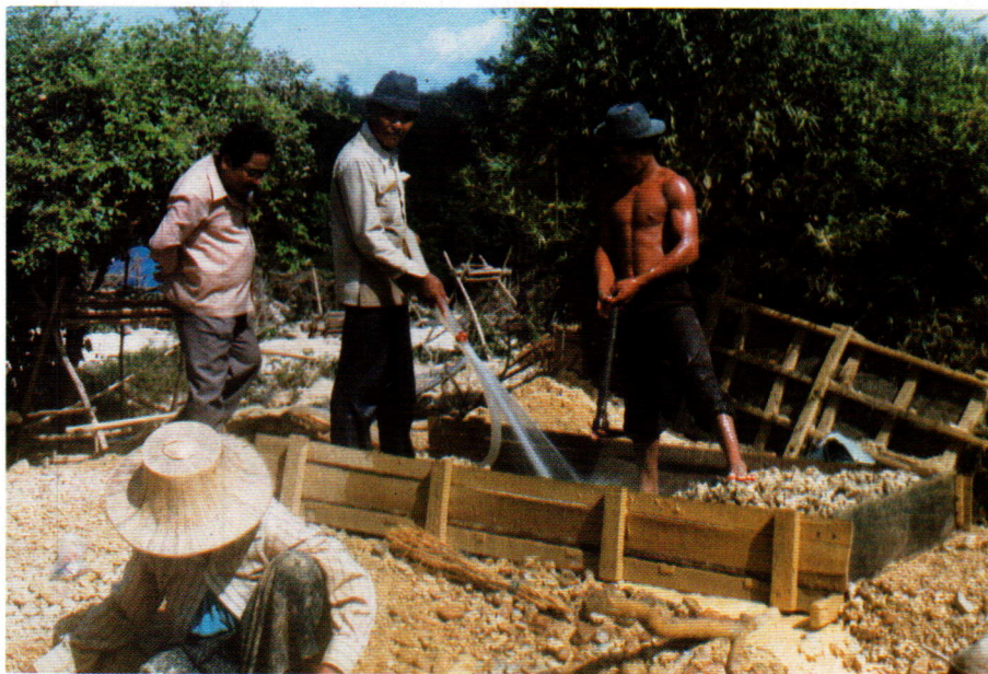
Sapphire mine at Bo Phloi, Kanchanaburi. Concentration of the sapphire-bearing gravel on the screens. Sand and clay are washed off by a water cannon.
