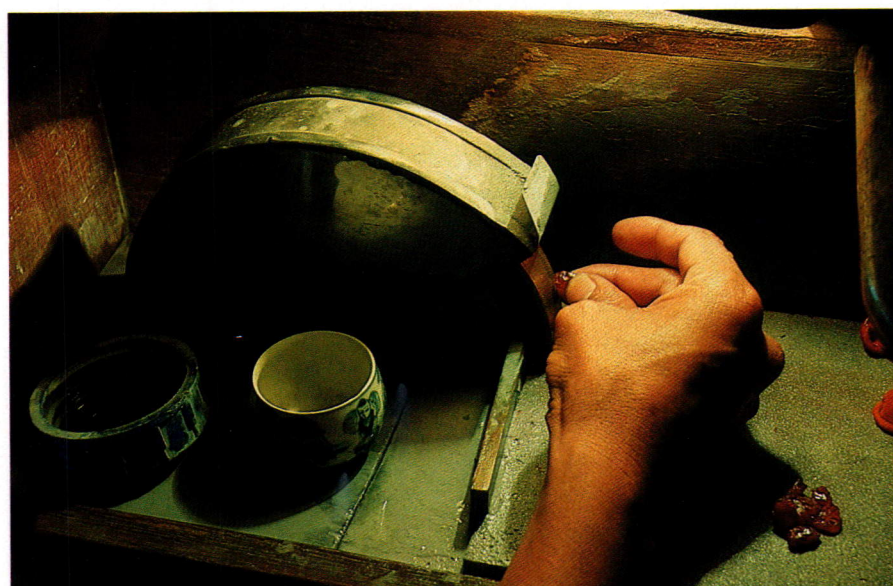
Grinding the gem to shape before cutting
