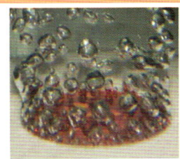
Low heat flux nucleate boiling
