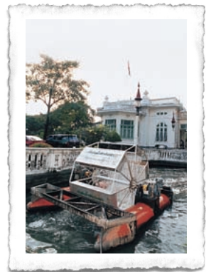
The Chaipattana Aerator in action at Phra Mongkutklao Hospital, Bangkok.
