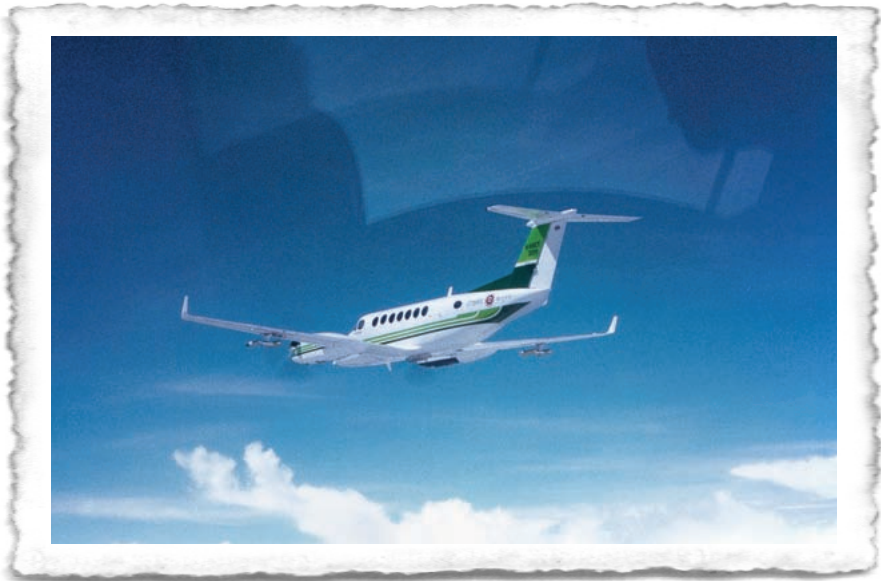
The Super King Air 350 used in the Super Sandwich technique of bombarding the rain clouds.
